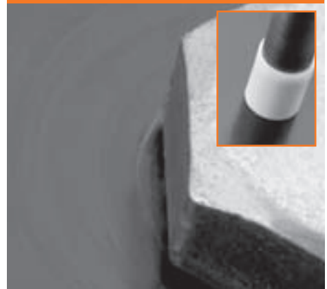
Static covered socket – Light Damage
