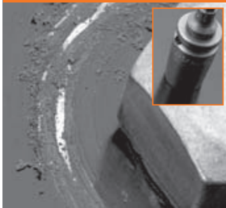
Standard socket – Heavy Damage
